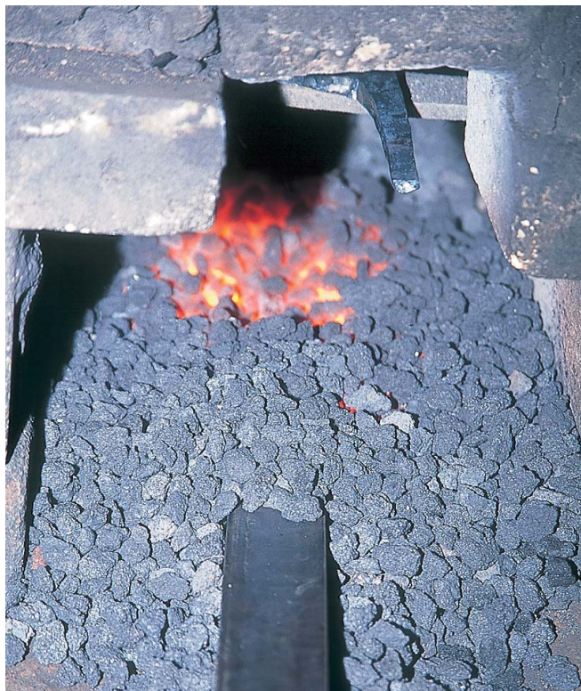
鉄を焼き上げる Steel is placed in the fire
